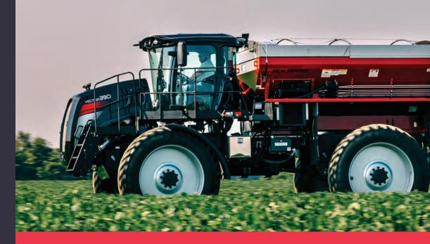
PRESSURE COMPENSATED HYDRAULICS HELP MAINTAIN RATES, EVEN AT LOW ENGINE RPMS.
